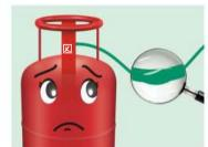
Check rubber tube regularly for leaks. Change tube every two years
