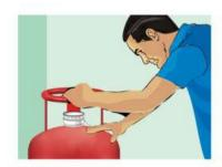
At the time of delivery, check whether the Company Seal and Safety Cap is intact
