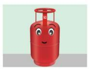
Always place cylinder at ground level, on a flat surface, and in a vertical position
