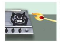
When lighting burner, strike match before switching on burner
